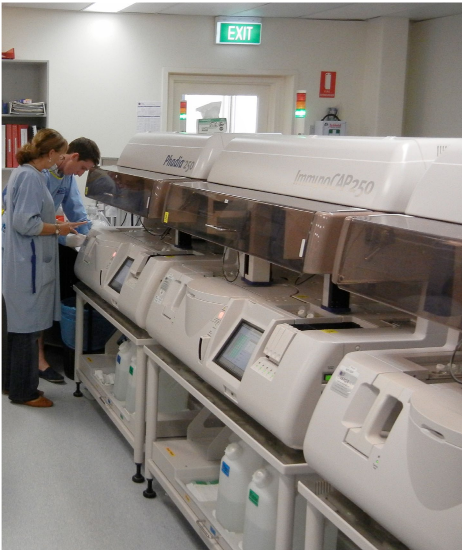
Faecal calprotectin testing at Sullivan Nicolaides Pathology's Immunology Department using a Phadia ImmunoCAP 250 immunoassay analyser
